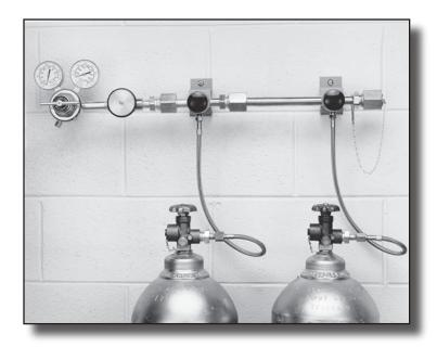
The 631 Series Simplex combines a modular manifold system with the extra heavy-duty 6700 Series regulator. Line or station regulators should be installed at the point of use to ensure constant delivery pressure. Use of Acetylene requires flashback arrestor on pigtails. All fuel gases require flashback arrestors.
