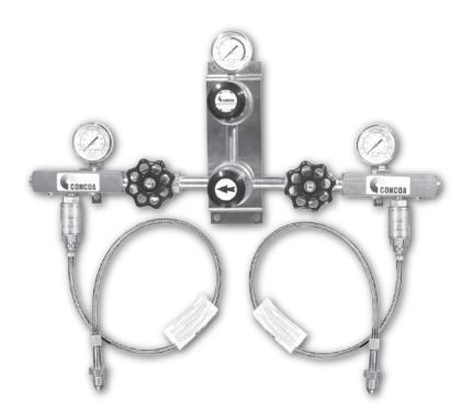
The 632 Series pressure differential switchover has been designed as a cost effective solution for high flow applications. With simple priority valve operation the 632 delivers 15, 50 or 120 psi output at flow rates exceeding 5,000 cfh. The simplistic design exceeds the stringent requirements for oxygen-acetylene NFPA 51 standards. Options include 1000-watt heaters for CO<sub>2</sub>, Advantium alarms and Intrinsic Safety Barriers for hydrogen service.
